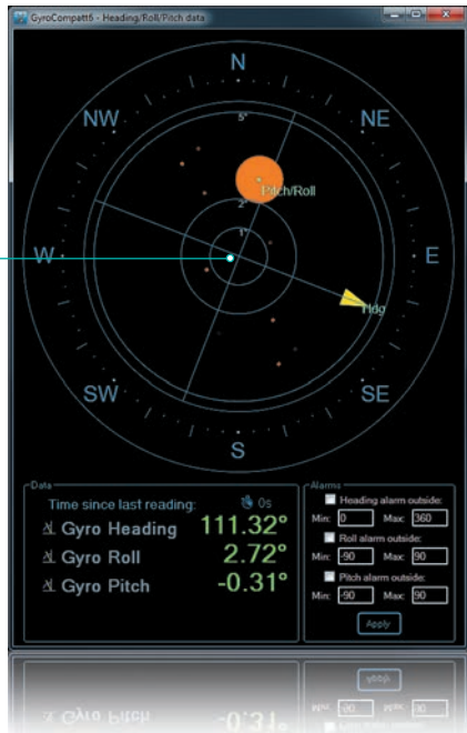
Bubble display for Gyro and Inclinometer
