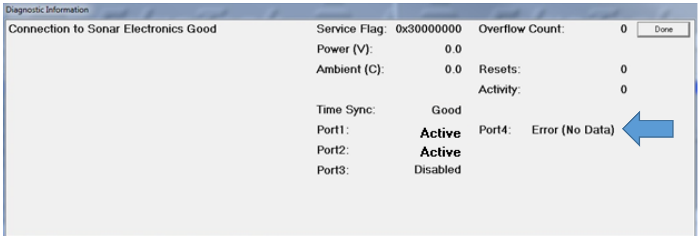
Figure 8-1: No Sound Velocity on Port 4
