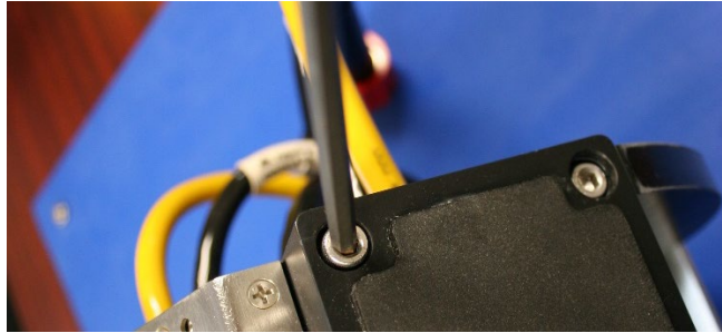
Figure 5-9: Remove the [6] Cap Screws
