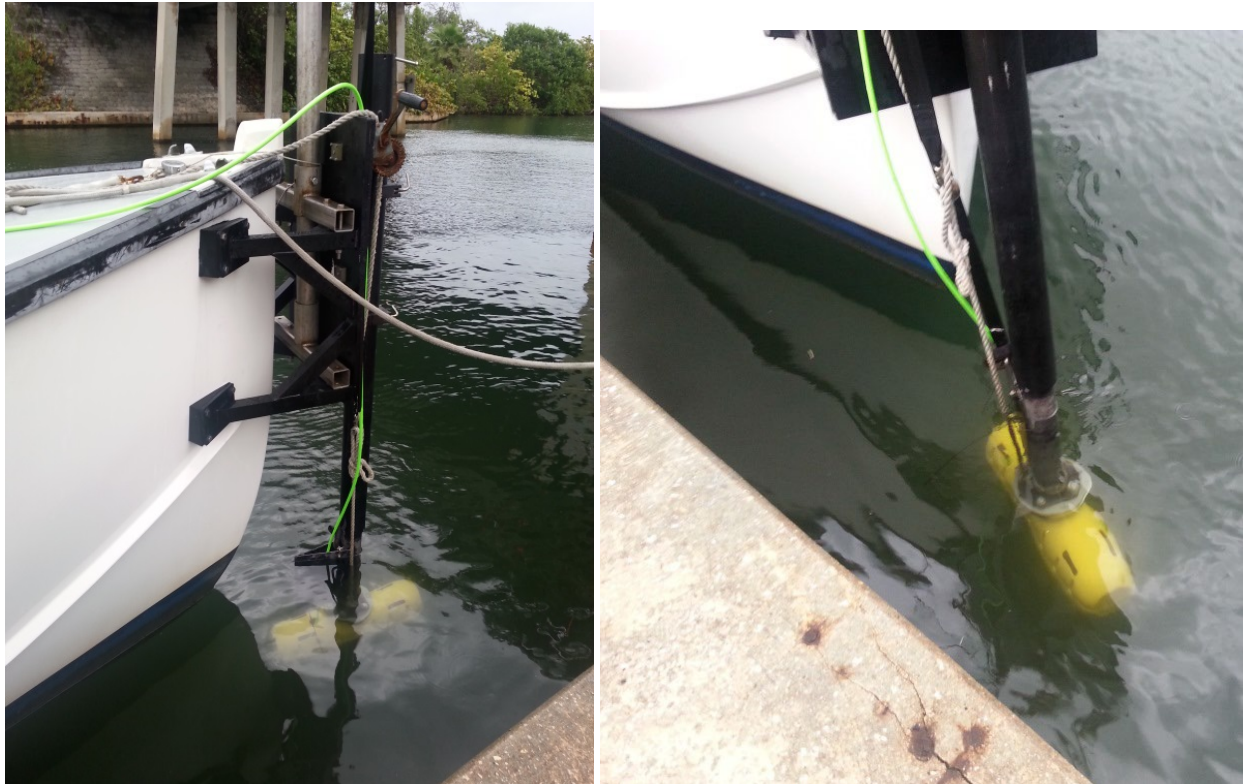
Figure 5-1: 6205s Deployment, Option 1 – Over-the-Bow
