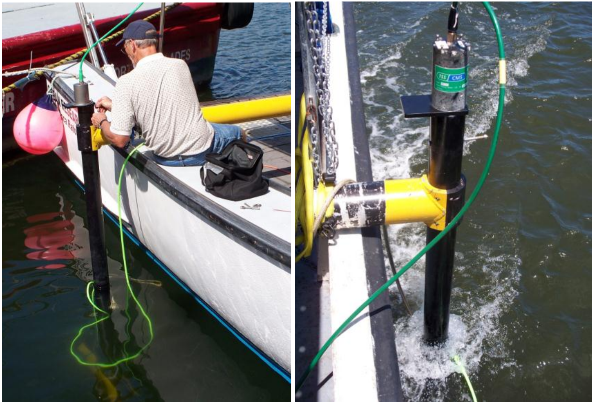
Figure 5-2: 6205s Deployment, Option 2 – Over-the-Side
