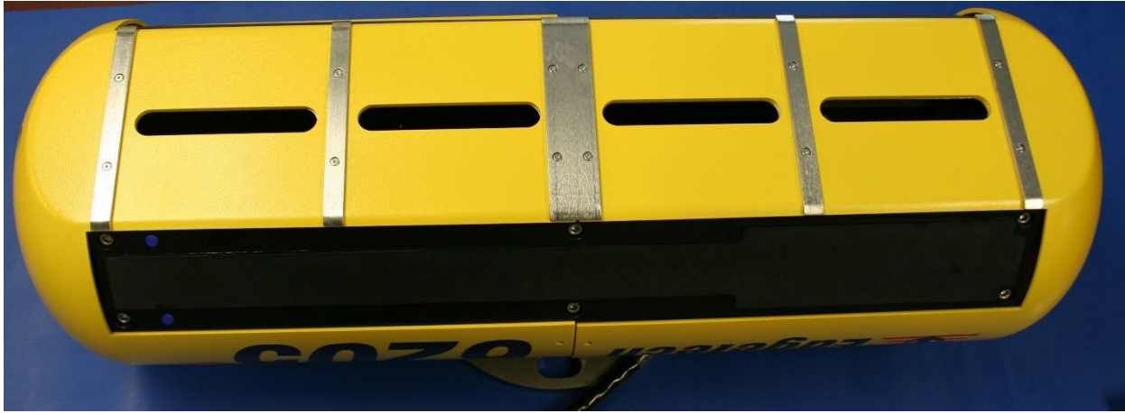
Figure 5-5: Top Housing and Deck Cable Removed
