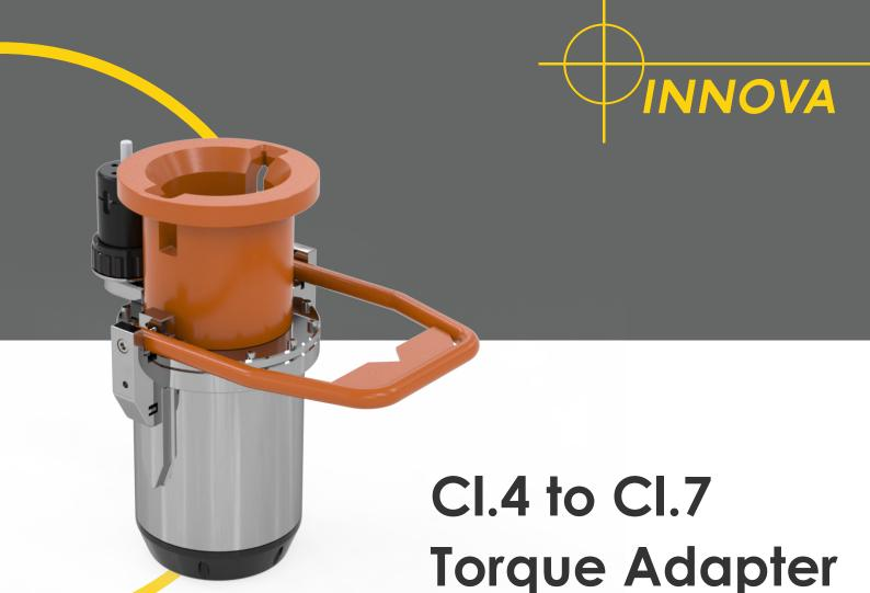
The Cl. 4 to Cl. 7 Torque Adapter is a gearbox for operating API 17H Class 7 interface valves with a Class 4 torque tool or actuator. The adapter can be provided with materials suitable for permanent installation subsea.
