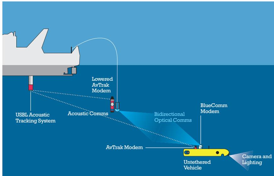
**Tetherless Vehicle Command and Control**
