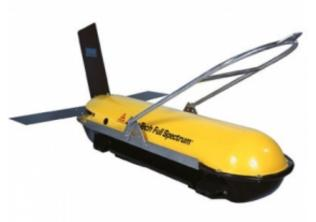
This is an integrated modular underwater sonar-mapping package designed for installation on a Remotely Operated Vehicle (ROV). It gathers side scan and/or subbottom data using EdgeTech's proprietary full spectrum chirp technology in water depths of up to 3000 meters.
