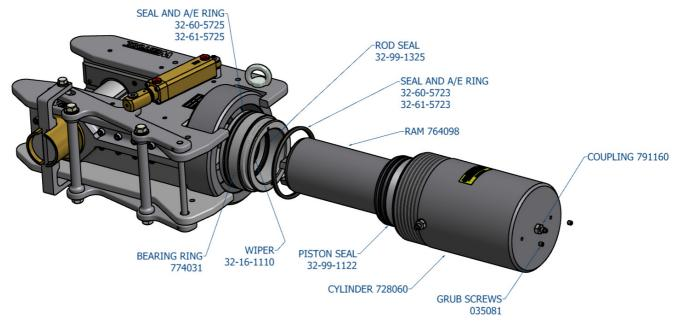
Put the assembled parts into a plastic dust bin or similar vessel, fit the coupling to the top of the cylinder, attach a hand pump to the coupling and pump out the ram, importantly, **by hand.** The ram will now be free of the cylinder and all seals will be accessible.
