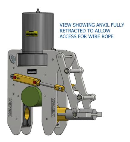
Operate the auxiliary cylinder instroke to position the anvil fully home under the wire rope, the main ram should not be activated until the auxiliary cylinders are operated to the full extent of their stroke.
