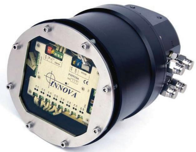
The Innova Quattro is an ultra-compact hydraulic controller unit with 4 valves each capable of providing up to 22 lpm hydraulic flow, proportionally controlled over a serial line. The system is ideal for controlling hydraulic tooling, such as torque tools, inspection tools etc, and generally for increasing the capacity of any ROV or tooling system in a simple manner.
