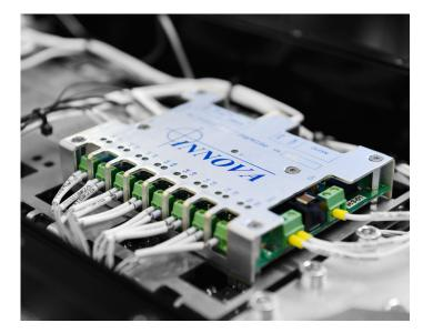
Control of proportional valves is provided by 16 channels of pulse width modulated output.
